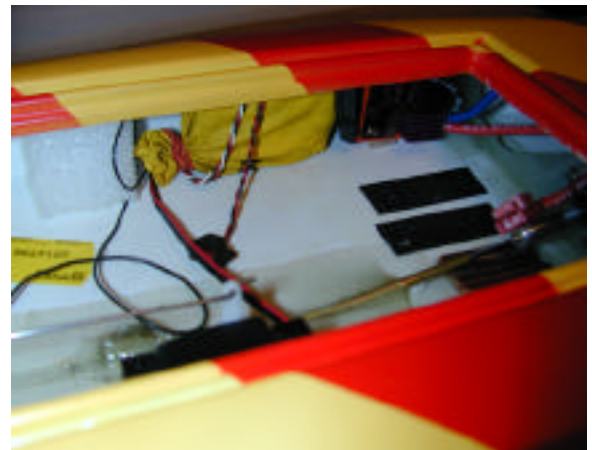
Receiver and ESC
